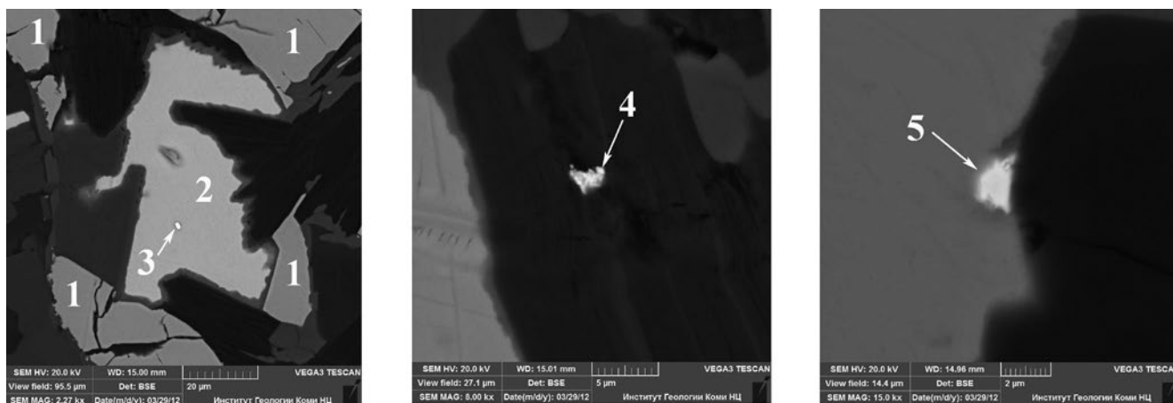
Fig. 1. Noble metal minerals in clinopyroxenites and hornblendites. 1 – magnetite, 2 – chalcopyrite, 3 – native gold, 4 – sperrylite, 5 – mertieite-II
