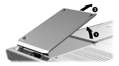
6. To remove the hard drive, pull upward on the hard drive tab **1** to release the hard drive, and then lift the hard drive **2** out of the hard drive bay.
