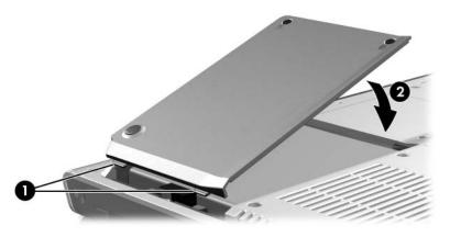
3. Tighten the 2 hard drive security screws.
