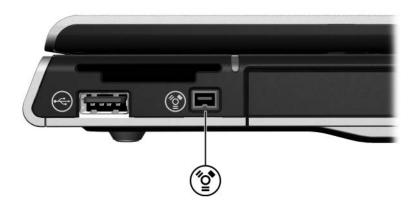
**CAUTION:** To prevent damage to the 1394 port connectors, use minimal force to insert a 1394 device.
