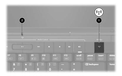
You can enable and disable the wireless devices with the wireless button. You can also enable and disable the wireless devices in the Setup Utility.
