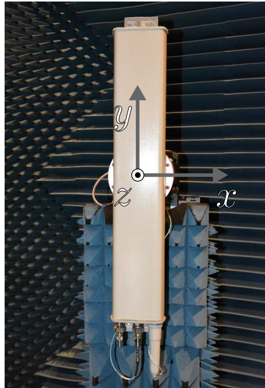
Figure B.1: BTS antenna mounted in IHF chamber.
