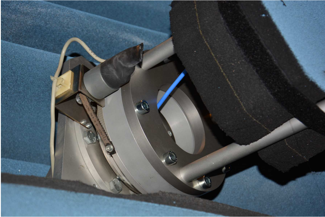
Figure 7.7: Probe displaced by \lambda/4 with additional spacer.
