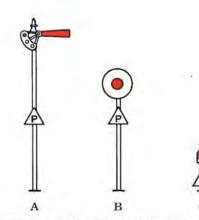
Indication: STOP. INSPECT TRAIN, TRACK OR STRUCTURE AS PROVIDED IN SPECIAL INSTRUCTIONS, AND PROCEED THROUGH REMAIN-DER OF THE BLOCK IN ACCORD-ANCE WITH PROVISIONS OF RULE 507, 663, 744, OR 776, AS THE CASE MAY BE
