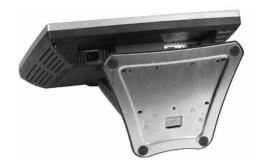
**4** Connect the power cord to the power connector under the bottom of the screen.
