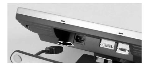
**5** If your computer supports analog video, connect the analog video cable to the analog connector under the bottom of the screen.
