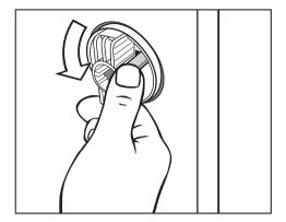
■ Release the catch and turn the right hand shipping strut counterclockwise by 90°.
