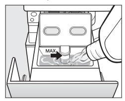
■ Add the fabric softener or liquid starch to compartment ��. Do not exceed the Max. level mark.
