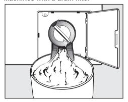
■ Place a suitable container under the access flap.
