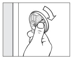
■ Release the catch and turn the left hand shipping strut clockwise by 90°.
