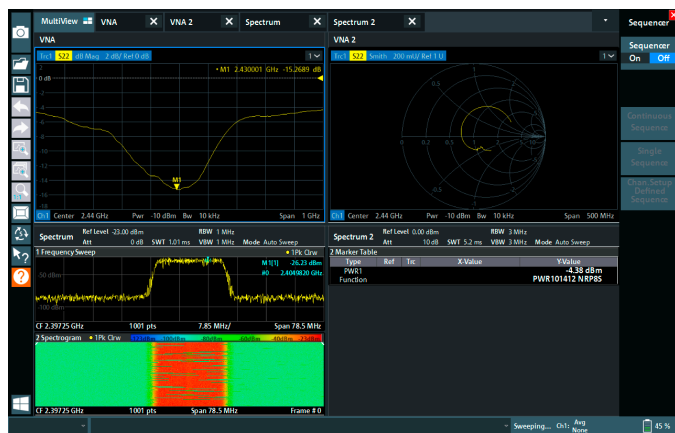
MultiView provides a convenient overview of all active R&S®ZNL modes. The figure shows a combination of spectrum analyzer and network analyzer. In this view, all modes can be updated sequentially.
