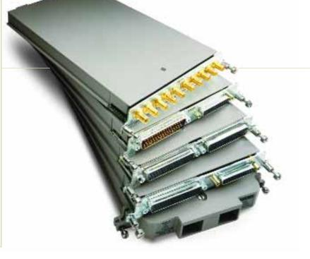
Use any combination of Series 7700 modules both matrices and multiplexers, just one type of module, or mix and match any combination. All modules function simultaneously.
