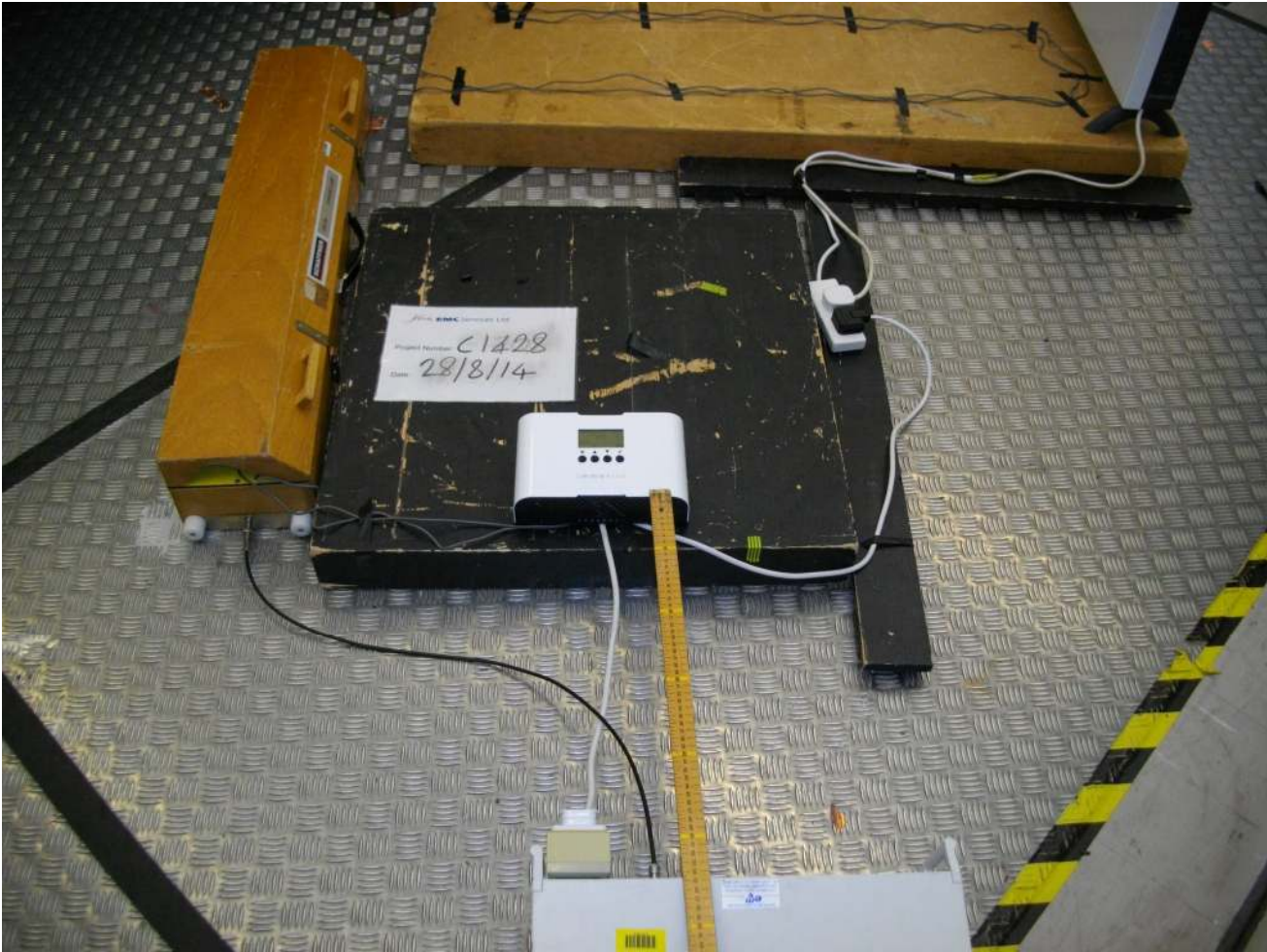
Photograph 5.16.9 Immunity to EFT/B testing
