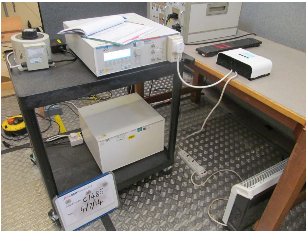
Photograph 5.16.3 Voltage dips and interruptions testing
