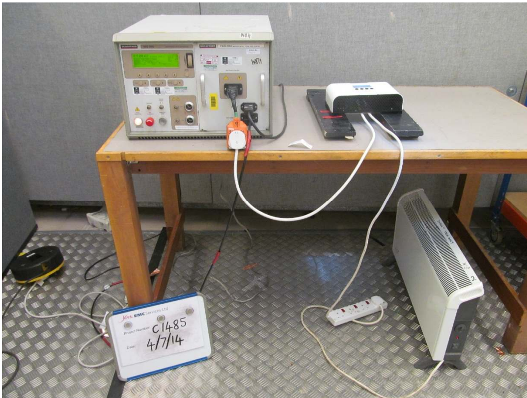
Photograph 5.16.5 Immunity to Surge testing
