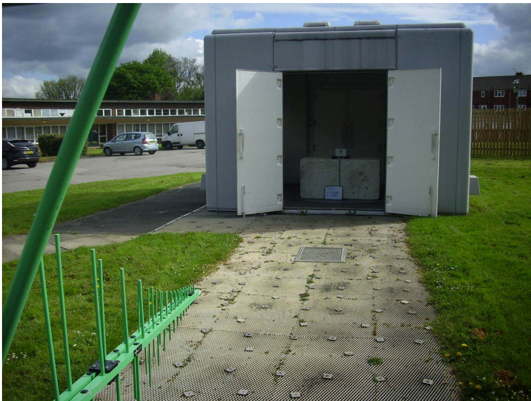
Photograph 5.16.1 Radiated emissions testing, 30MHz to 1000MHz
