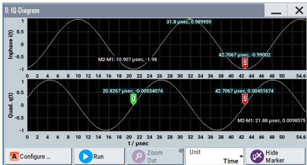
Figure 8-1: I/Q diagram with markers
