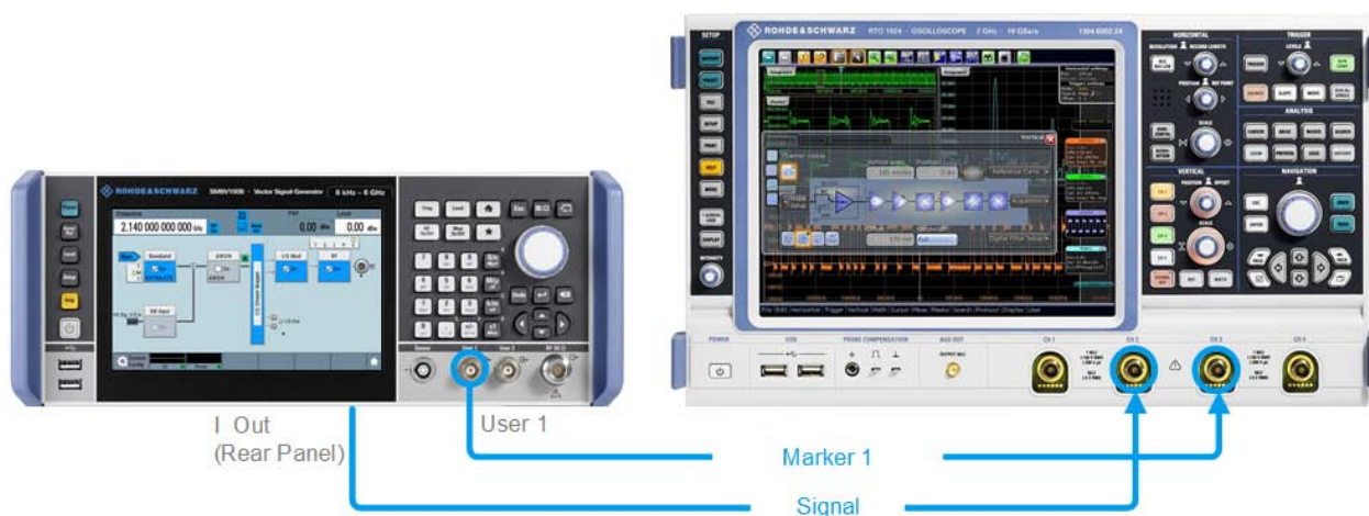
Figure 3-11: Simplified representation of a test setup for signal monitoring**
