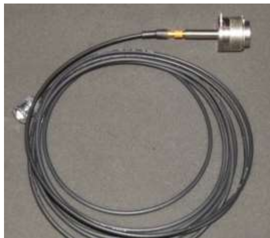
G.R.A.S. High Frequency Audio Coupler
