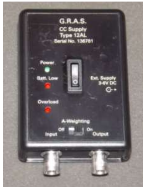
G.R.A.S. 12Al 1-Channel CCP Power Module
