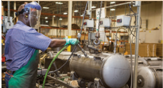
Every air compressor manufactured by Mi-T-M is tested after the final assembly stage
