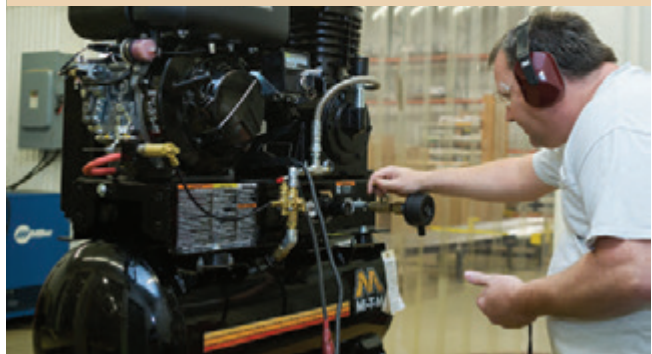
Every air compressor manufactured by Mi-T-M is tested after the final assembly stage
