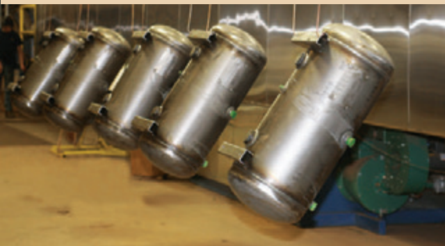
A 7-stage powder coating system applies superior finish that is harder and more durable than conventional paint
