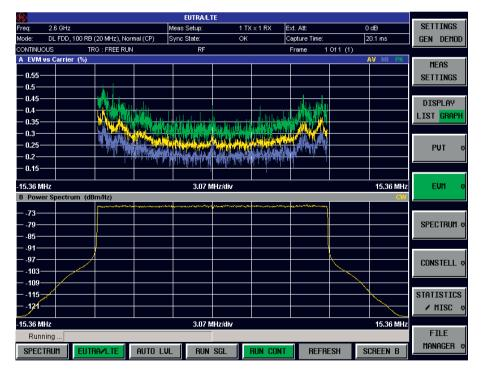
Analysis of a EUTRA/LTE FDD downlink signal with a bandwidth of 20 MHz.
