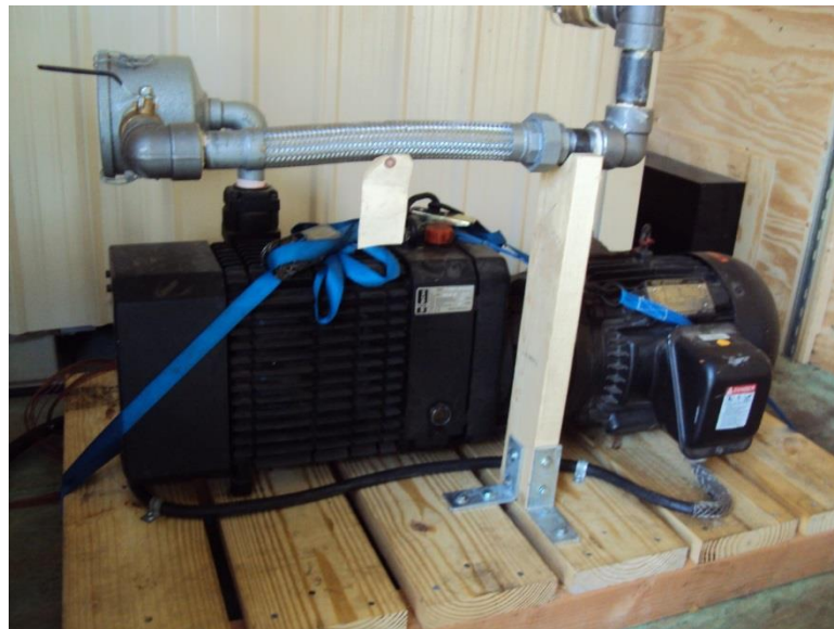
Figure 27. Busch Mink 7 horse power vacuum pump can remove about 56 cfm of air.
