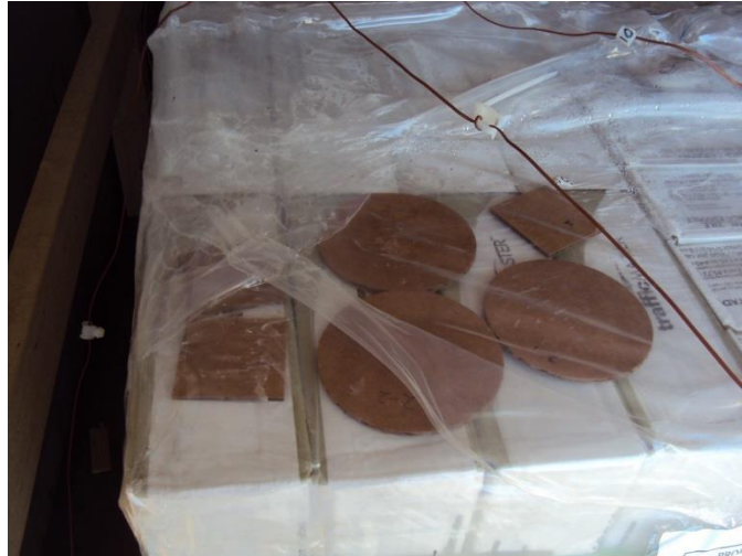
Figure 30. The corrugated paper boards were placed on the top of unit load of tiles.
