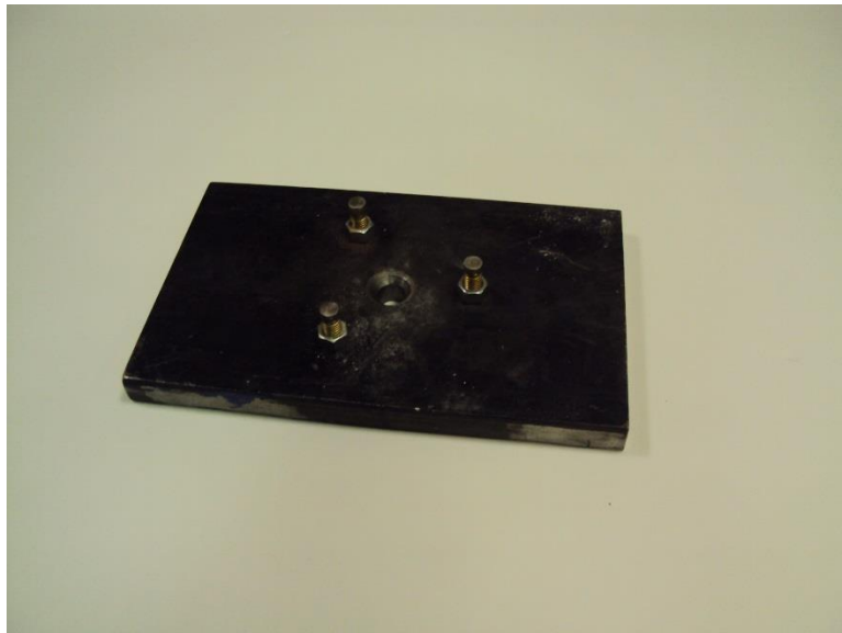
Figure 48. The equal-lateral triangular support made in the breaking strength test.
