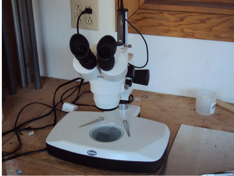
Figure 43. Motic light microscope (Motic SMC – 140) used to check snails for a heart beat
