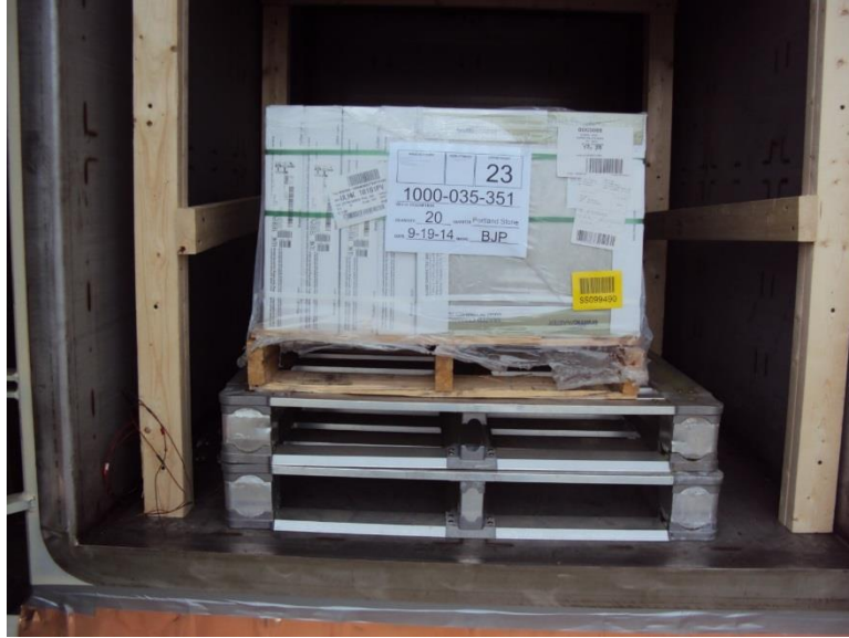
Figure 35. The unit load of tiles was set on two aluminum pallets inside the chamber.
