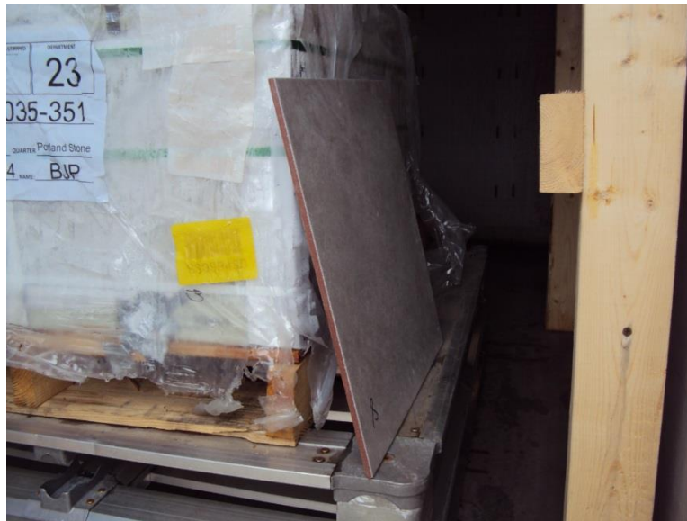
Figure 40. A ceramic tile was placed next to the unit load during the vacuum and steam treatment for later testing of properties.
