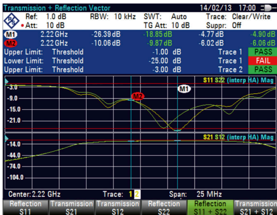
Vector network analysis: Simultaneous display of four S-parameters ( S_{11} , S_{21} , S_{12} , S_{22} )
