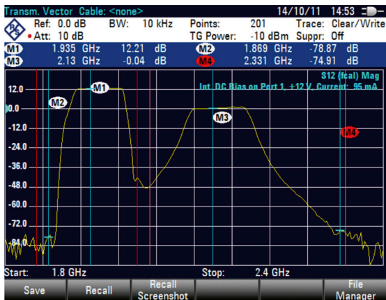
Two-port capability for transmission measurements
