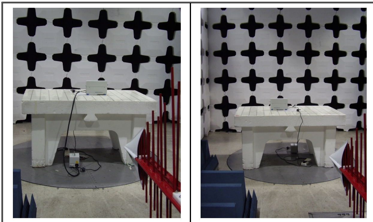
Picture # 3. Radiated emission test setup Front and rear views
