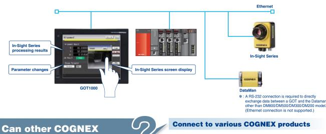
The In-Sight vision system and DataMan barcode reader can be connected to the GOT.
