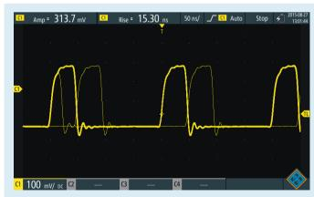
The high-speed acquisition system of the R&S°Scope Rider captures up to 50 000 waveforms/s and uncovers rare and unexpected signal anomalies.
