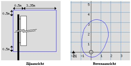
Figure NL-1. Calculation of the radiated fields by a base station's antenna.
