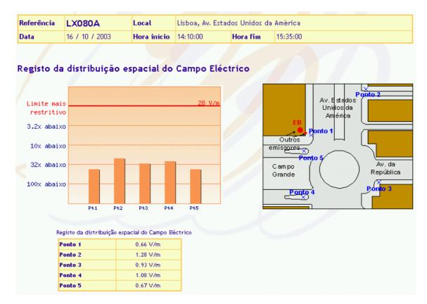
Figure POR-6. Results of a spot measurement. Several spots around the base station are chosen for a frequency selective measurement
