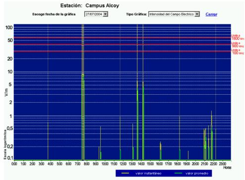
Figure SP-5. Plot of a daily monitoring showing the electric field strength compared with the limits of the guidelines (in red).
