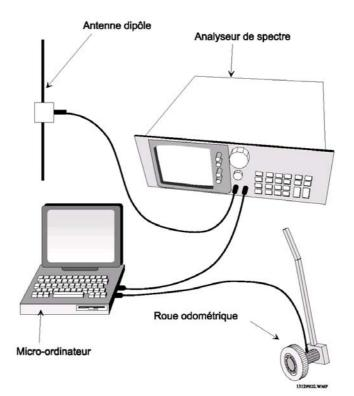
Figure BE-2. Scheme of the method used to measure EMF along a trajectory in ISSeP.
