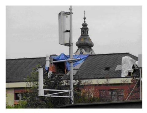
Figure AU-3. Broadband measurement station
