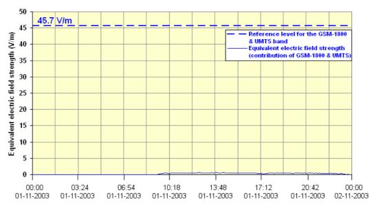
Figure GR-6. Variation of the electric field strength of the GSM 1800 and UMTS bands measured at a station during one day.
