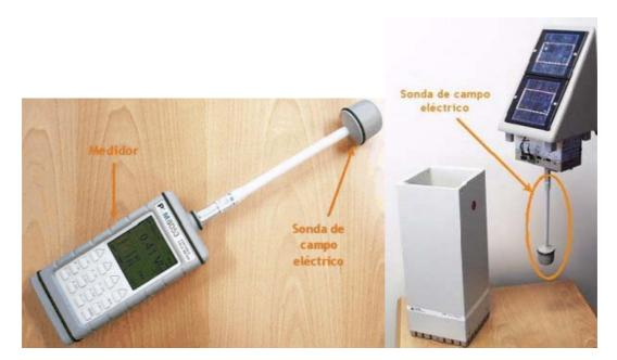
Figure POR-2 Portable and remote monitoring sets.
