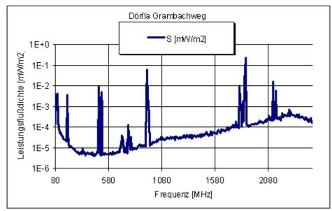
Figure AU-2. Values of spectral power density measured in Dörfla (Austria)
