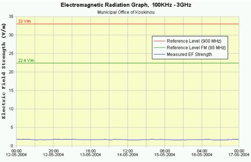
Figure GR-5. Electric field strength versus time at a monitored location of the project.
