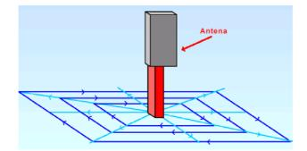
Figure POR-1. Maximum-radiation grid for an isolated antenna.
