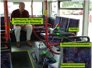
Figure GE-8. Measurement scenario in a bus.
