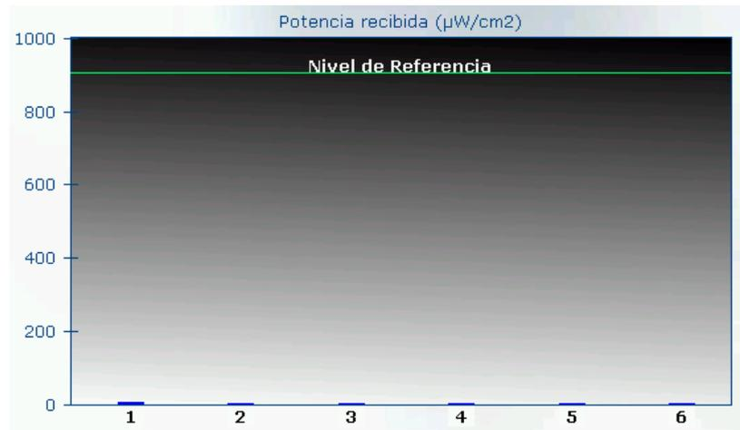
Figure SP-7. Graphical representation of the power density (Potencia recibida) of 6 spot measurements according to the distances (Distancia) shown in Table SP-2, i.e., the location 1 in this figure corresponds to the distance 3.7 m in Table SP-2.
