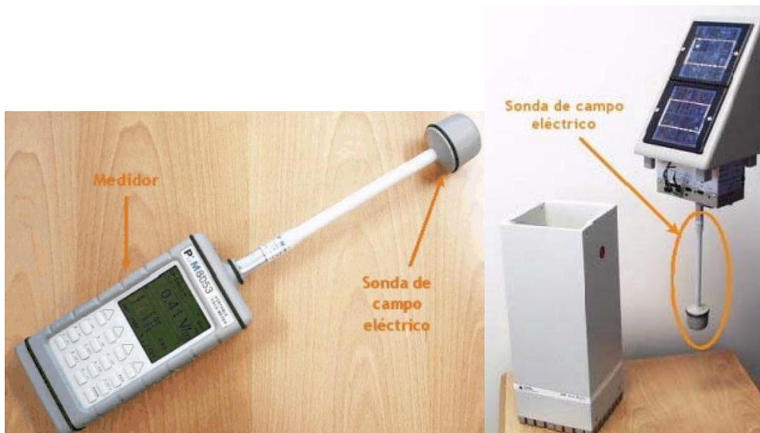
Figure POR-2 Portable and remote monitoring sets.
