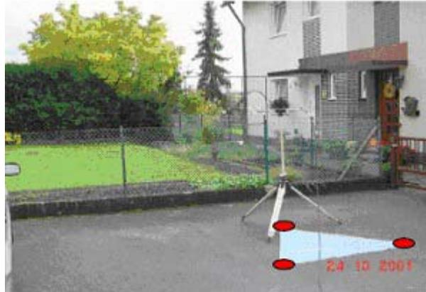
Figure GE-5. Typical measurement scenario: In red, the 3 measurement spots that form a triangle of 1.5 meter side.
