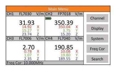
AR Field Monitors can display single-channel, multichannel, minimum and maximum, and average field-strength data.
