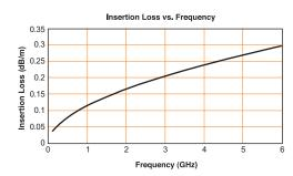
**CC5 Series:** Low-loss microwave cables designed for higher power applications with frequencies up to 11 GHz. VSWR typically less than 1.25:1.
