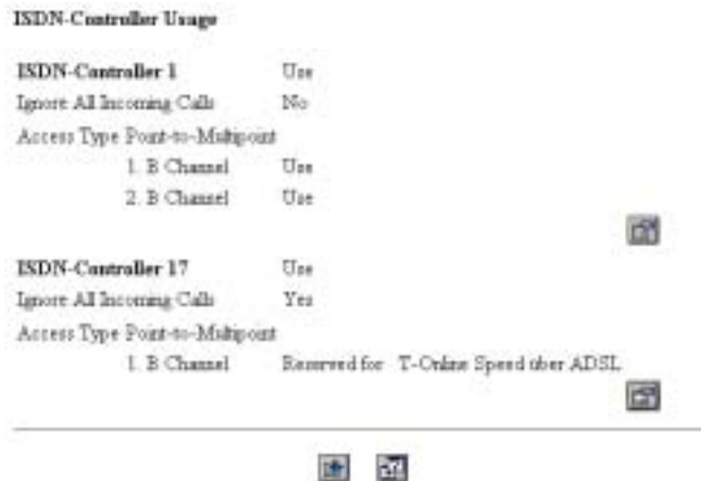
Settings for the ISDN-Controller 1 and the ADSL-Controller 17
