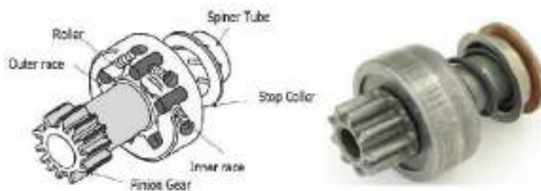
Gambar 2.25. Over running clutch dan pinion gear
