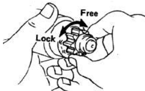
Gambar 2.71. Memeriksa pinion gear dan over running clutch
