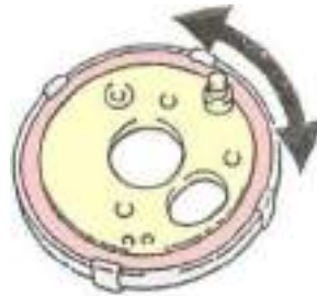
Gambar 1.90. Memeriksa breaker plate
