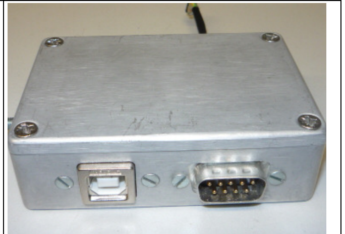
Figure 5: Detailed view of battery box with signal ports [Detailansicht der Batteriebox mit Signalanschlüssen]
