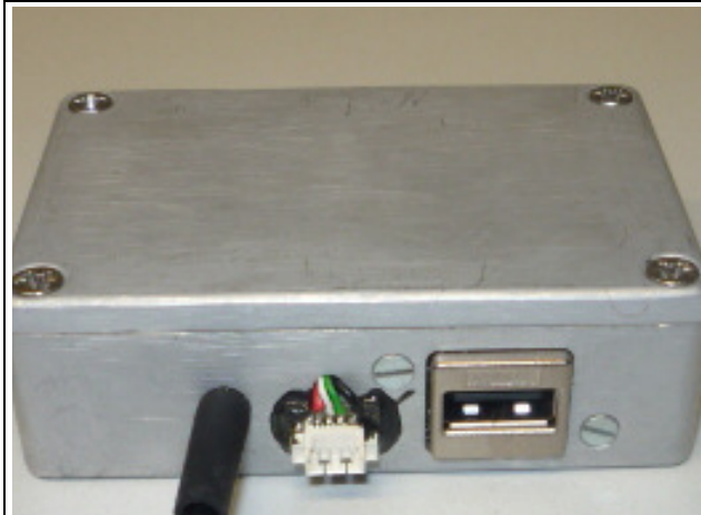
Figure 4: Detailed view of battery box with signal ports [Detailansicht der Batteriebox mit Signalanschlüssen]
