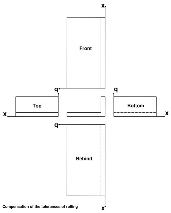
The reference of the dimension (for example "upper edge") indicates from which edge of the piece the dimensions are taken. That means that the eventual tolerances of rolling will be placed on the opposite. If we give no reference for the dimension, the previous value stays valid. The reference of the dimension does not modify the value of a coordinate, it is the post-processor which must uses it to balance the tolerance of rolling.
