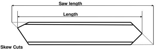
The skew cuts of the web are represented in the view of the front face, the ones of the flange in the bottom face.
