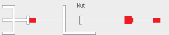
Adapter with BNC jack, specific for each CDN, e.g. with 3 banana plugs for CDN M3
