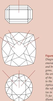
Figure 9: Diagrams of emerald-, cushionand brilliant-cut gems, showing the orientation of the gem facets to the light path /optical plane of the refractometer (as in Figure 7) for grazing illumination.
