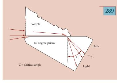
**Figure 4**: *Sketch of the light path in the sample and prism of a Pulfrich refractometer when solids are measured.*
