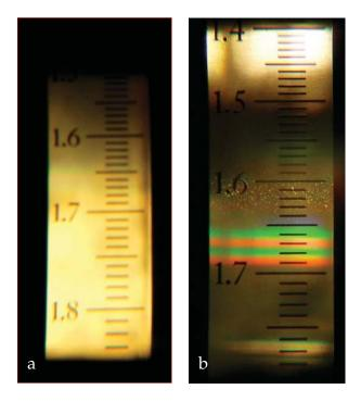
**Figure 8:** *Refractometer readings for a peridot when illuminated by white light with (a) traditional illumination, and with (b) grazing illumination.*
