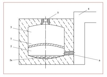
Figure 2: Cross-section of a single retort furnace for zinc white production at Olawa (Jasinski et al., 1987): (1) ceramic diaphragm; (2) vaporizing chamber; (2a) metallic zinc melt; (3) combustion chamber; (4) zinc vapour oxidizing chamber; (5) gas burner; (6) zinc vapour burner.
