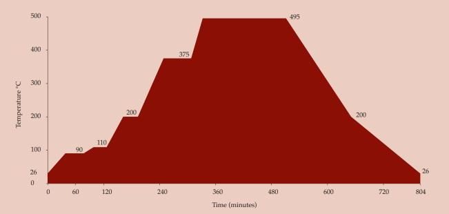
**Figure 2:** Chinese aquamarines are heated to 495°C at 3°C/min. in the stages shown. They are held at 90°C for 60 min., at 110° and 200° for 30 min. each, at 375° for 60 min. and at 495° for 180 mins.
