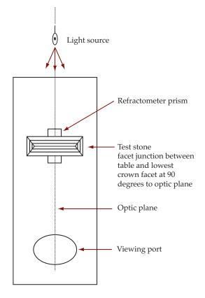
**Figure 7**: *Diagram of a refractometer showing the placement of a gem with respect to the optic plane of the refractometer.*
