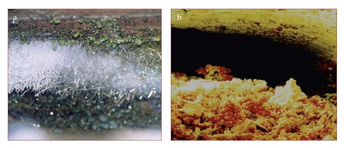
**Figure 3**: *Zincite crystals in vaporizing chamber: (a) on roof of chamber; (b) fallen crystals on floor of chamber. Photographs by R. Jaslan.*
