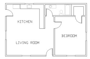
**Figure 16-27:** A floor plan of an apartment drawn using multilines. Thanks to Bill Wynn of New Windsor, Maryland, for this drawing.
