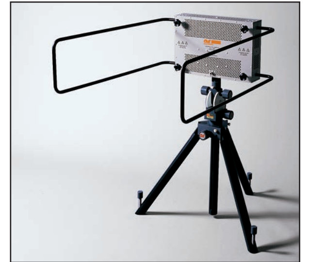
FIELD STRENGTH MEASURED BETWEEN TYPE A ELEMENTS
