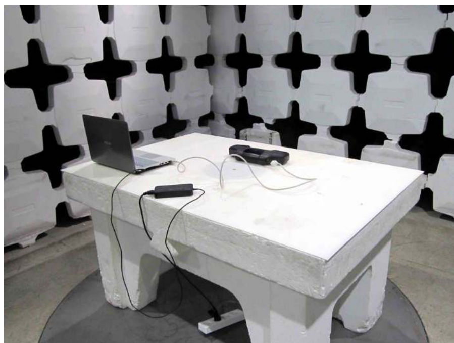
Picture # 4. Radiated emission test setup. Normal operation
