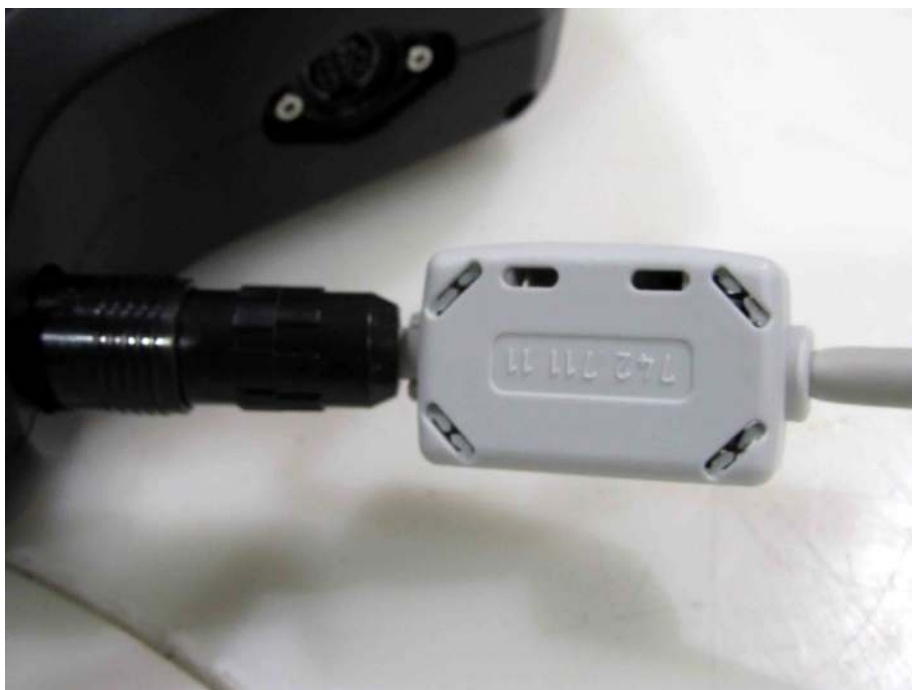
Picture # 6. Normal operation. Ferrite on external USB cable
