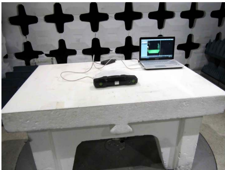
Picture # 5. Radiated emission test setup. Normal operation
