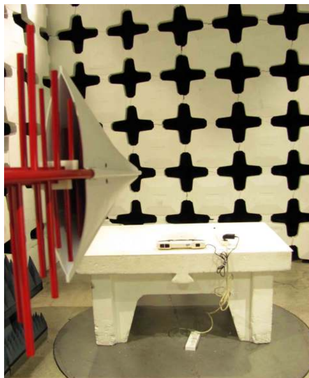
Picture # 8. Radiated emission test. Charging w. FRIWO Charger
