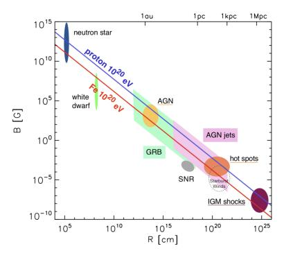
**Figure 8.** Updated Hillas diagram [7], obtained by requiring the Larmor radius for a  $10^{20}$  eV particle to be smaller than the characteristic source size *R*. The blue line and the red line show the limits for protons and iron nuclei, respectively. Shown also are astrophysical objects that can meet the requirements on source size and magnetic field *B* (above the respective lines). AGN (radio galaxies) typically represent suitable environments. Adapted based on ref. [4].
