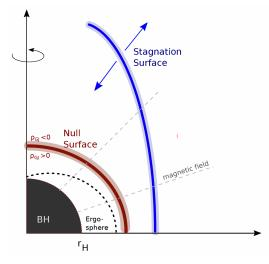
**Figure 11.** Illustration of possible locations of charge-deficient regions (gaps) around a rotating black hole in which UHECR acceleration could occur. The red line denotes the null surface across which the required Goldreich-Julian charge density  $\rho_{GJ}$  changes sign, while the blue line delineates the stagnation surface from which stationary MHD flows start.
