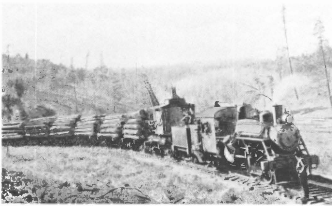
FIGURE 1.27. Logging train in New Mexico's Sacramento Mountains near Cloudcroft. The locomotive is a geared, Heisler type. The log loader, here just behind coal tender, was steam powered, and traveled from car to car on rails. To unload, the process was reversed, hence the need to bring the loader along in the consist (from postcard collection of Spencer Wilson).
