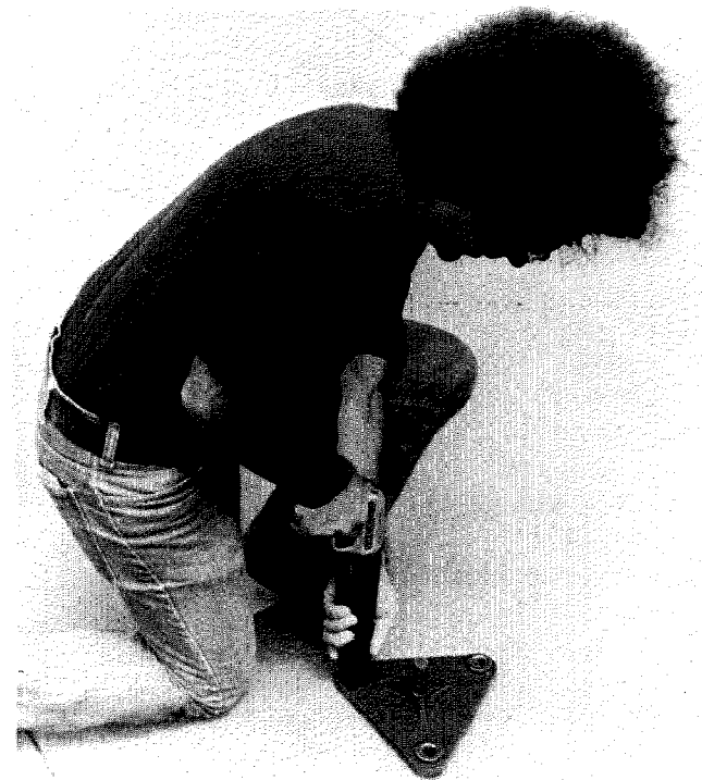
FIGURE 12. Windsor probe in use.
