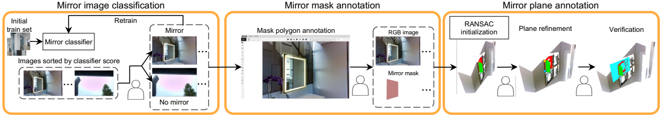
Figure 2: Our human-in-the-loop mirror mask and 3D plane annotation workflow. We leverage an iteratively trained mirror image classifier to assist a user in rapidly selecting all mirror images in an input image dataset. The images are then annotated with mirror surface polygon masks. The masks and their corresponding depth images are used to initialize mirror plane estimates with a RANSAC approach. The user then refines and verifies all 3D mirror plane estimates.
