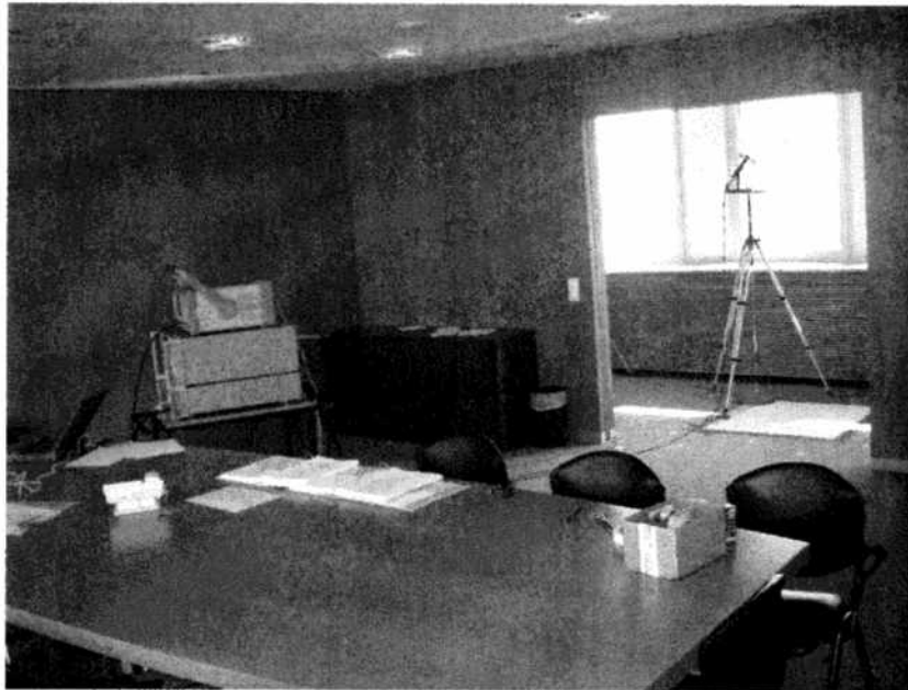
Figure 4: Picture of the conference room and the anteroom with the measurement antenna, the reference antenna can not be seen, it is far left behind the wooden wall. The two spectrum analyzers and the Notebook were in the conference room (for the measurements of GSM 900, DCS 1800, UMTS and UHF - ORF2).
