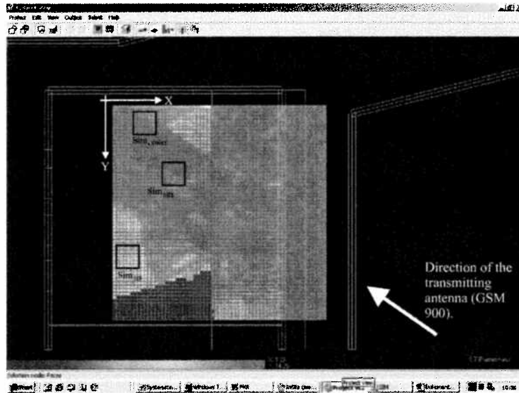
Figure 169: Schematic of the three cubes on specific locations within the simulated volume. Cube Sim_{CONST} is located in a region with field strength values in nearly the same range, Cube Sim_{HS} is located in a region with lower field strength values and a small region with higher field strength values ("Hot Spot") and cube Sim_{MIX} is located in a region with both, higher and lower field strength values.
