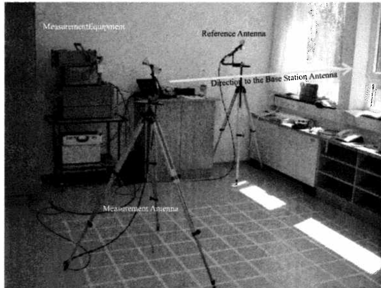
Figure 103: Picture of the measurement antenna, the reference antenna, the measurement equipment (spectrum analyzers and Notebook) and the grid. The grid steps of 25cm was taped on the floor.
