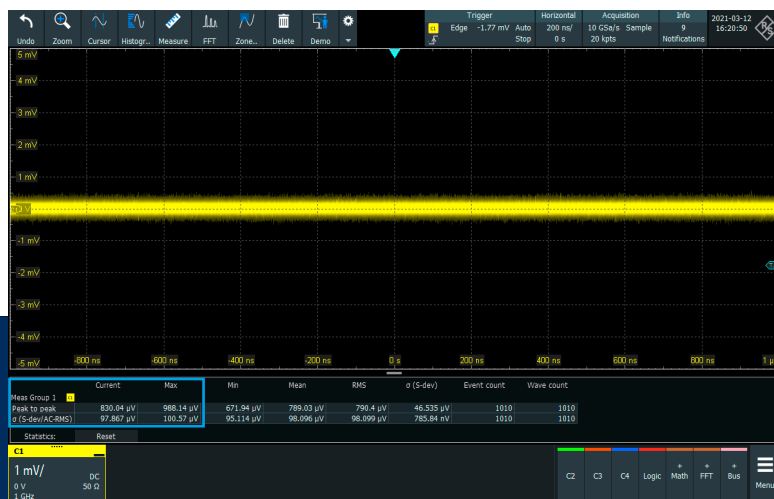
R&S®RT06: 100 μV (RMS) at 1 GHz bandwidth, 1 mV/div
