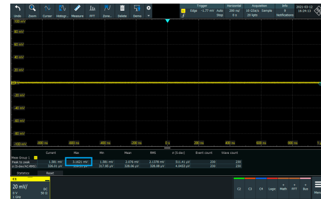
20 mV/div (noise V_{pp} = 3.16 mV)
