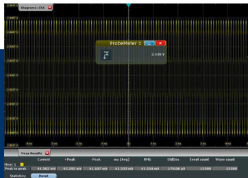
Using built-in probe offset (3.0 V rail at 2 mV/div, V_{pp} = 14 mV)
