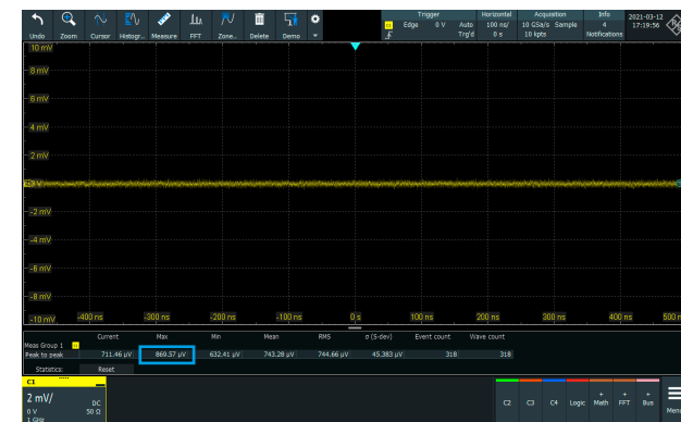
2 mV/div (noise V_{pp} = 870 \mu V)
