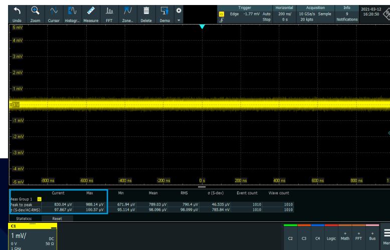
R&S®RT06: max. 988 μV ( V_{pp} ) at 1 GHz bandwidth, 1 mV/div
