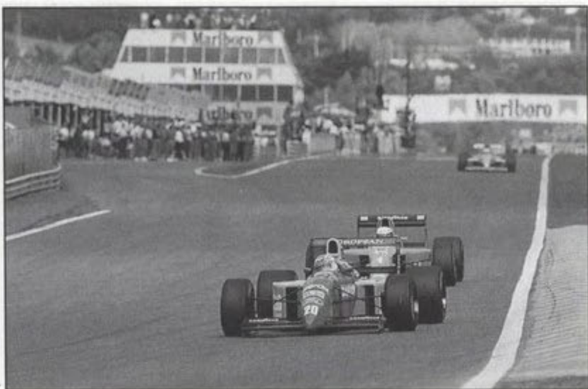
The rear car 'slipstreams' the car in front of it on the straight in the Portugese Grand Prix; 'getting a tow' prior to overtaking.
