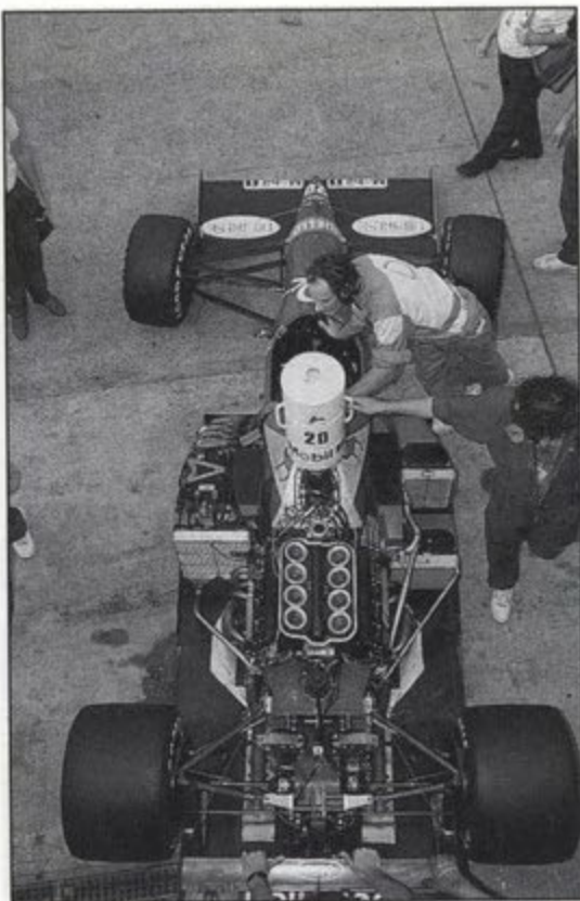
Re-fuelling the Benetton car at Hockenheimring. A F1 car holds 200 litres of 102 octane fuel and consumes 1 litre every 1,600 metres.
