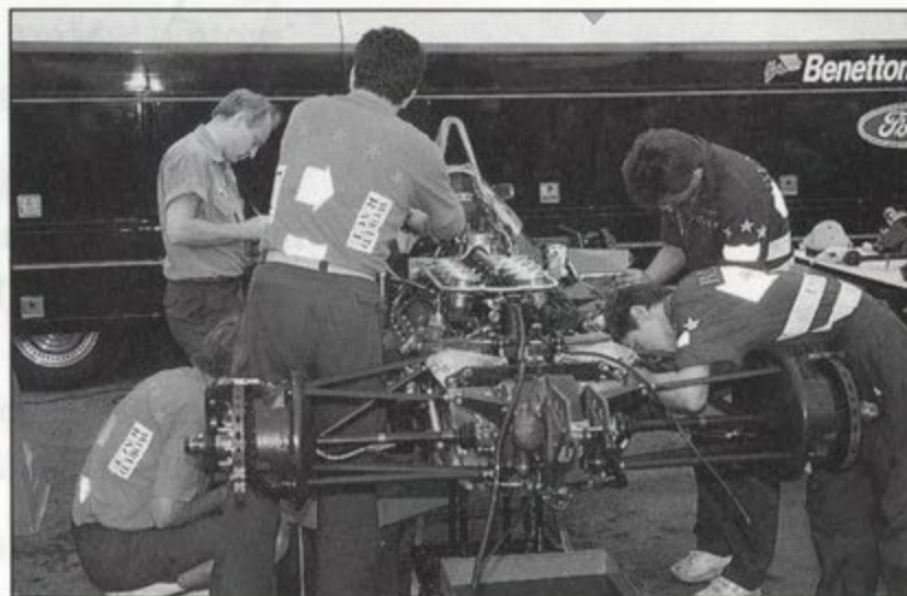
A stripped down Benetton B188 jacked up to give the mechanics good access to the rear suspension unit.
