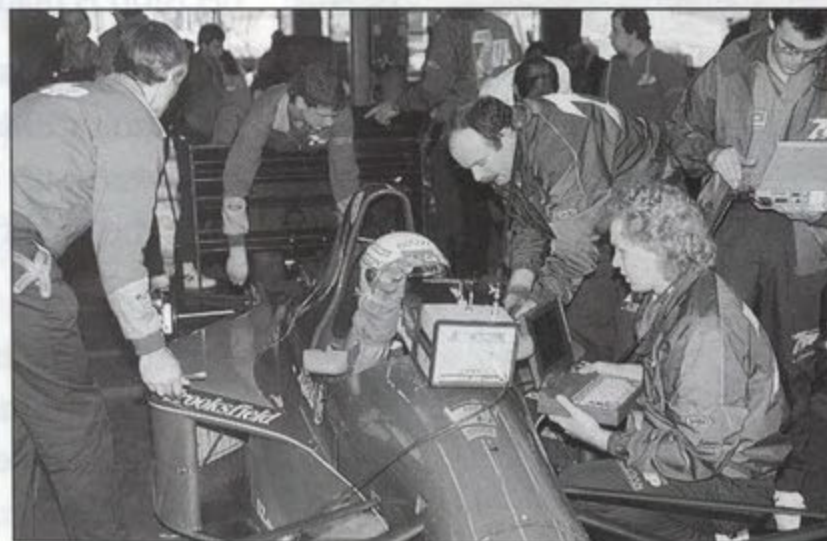
The driver and technicians of the Jordan team look at the data recorded by the telemetry system over a previous qualifying lap to help set the ideal gear ratios for the Phoenix circuit.
