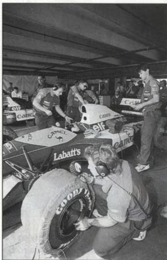
Race mechanics complete their checks on Nigel Mansell's car at Phoenix. The tyreman makes sure the blankets have raised the working temperature of the tyres.
