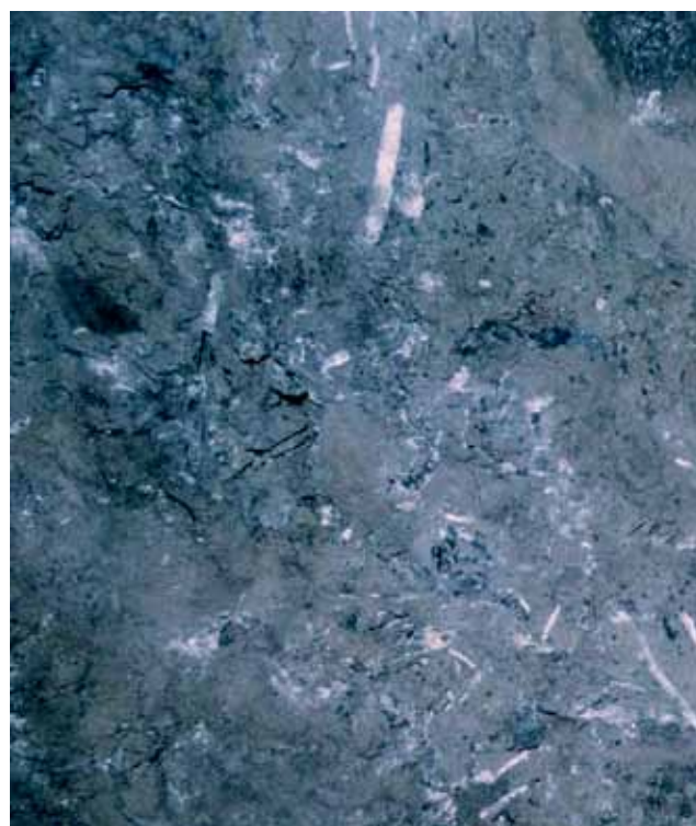
Figure 10. Baryte crystals embedded in a silt-like rock. Field of view approx. 0.5 m.
