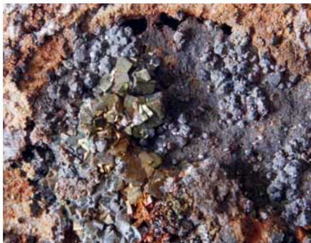
Figure 20. Cubes of pyrite with minor oxidation coating in places. Field of view 35 mm.
