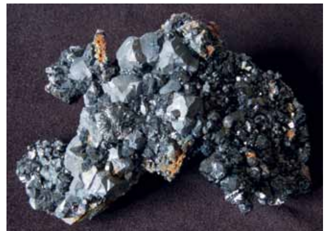
Figure 18. Cubo-octahedral galena crystals with sphalerite and minor goethite and quartz. Specimen width 14 cm.
