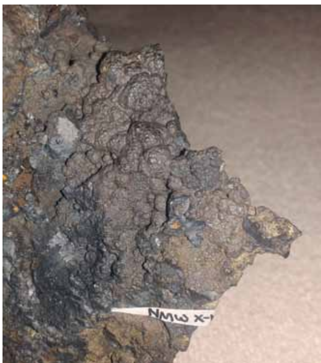
Figure 4. Botryoidal cryptomelane. Manganese trials at Gyrn Ddu. Field of view 4 cm tall. National Museum of Wales Collection No. NMW 2007.16G.M.2.
