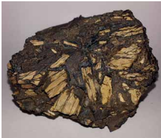
Figure 3. Grey to black, botryoidal manganese oxides (probably cryptomelane), cementing brecciated bleached mudstone. Manganese trials at Gyrn Ddu. Specimen 6 cm tall. National Museum of Wales Collection No. NMW 2014.11G.M.11.
