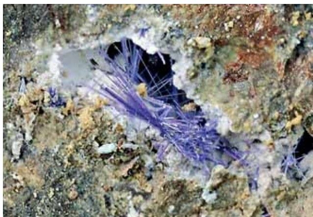
Figure 2 Cavity in cerussite-rich veinstone, lined with hydrocerussite (white) and a sheaf of distinctive, purple acicular elyite crystals (length 1.5 mm). Specimen: J.S. Mason Collection.
