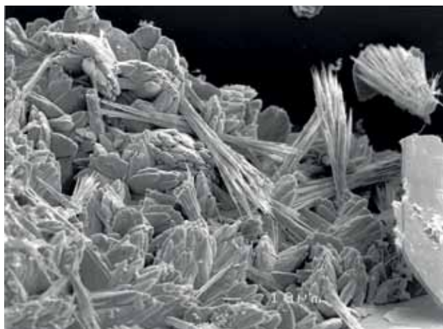
Figure 9. Mottramite crystals, from Mottram St Andrew, Cheshire. The acicular crystals are malachite. (SEM photo; scale bar 100 \mu\text{m} ).
