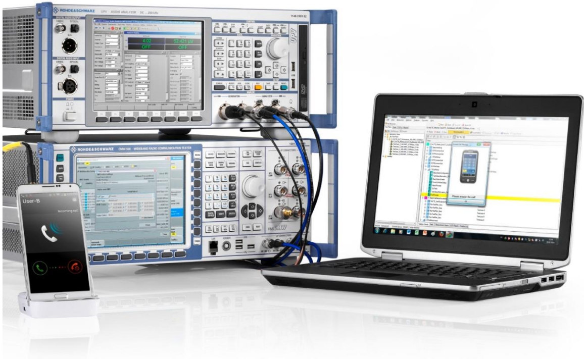
Fig. 2-2: VoLTE test setup with CMW500 and UPV
