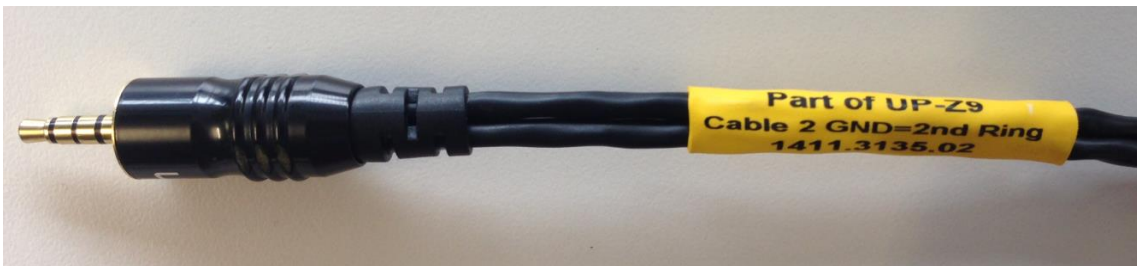
Fig. 7-4: Cable 2 GND=2 nd Ring, part no.: 1411.3135.02
