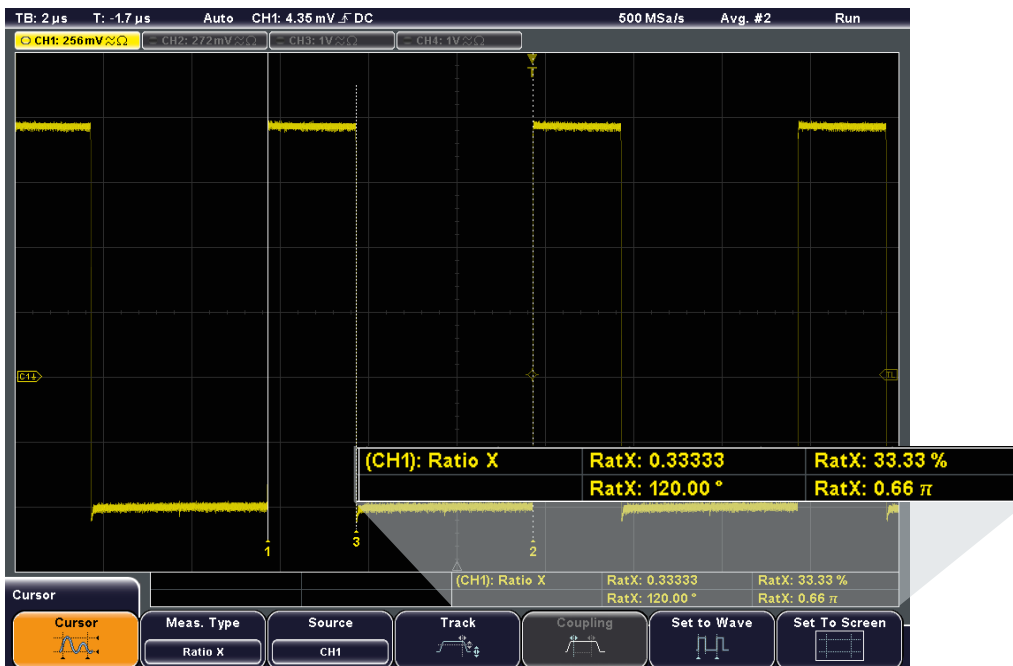
Special cursor measurement: using three cursors to determine the duty cycle of a pulsed signal.
