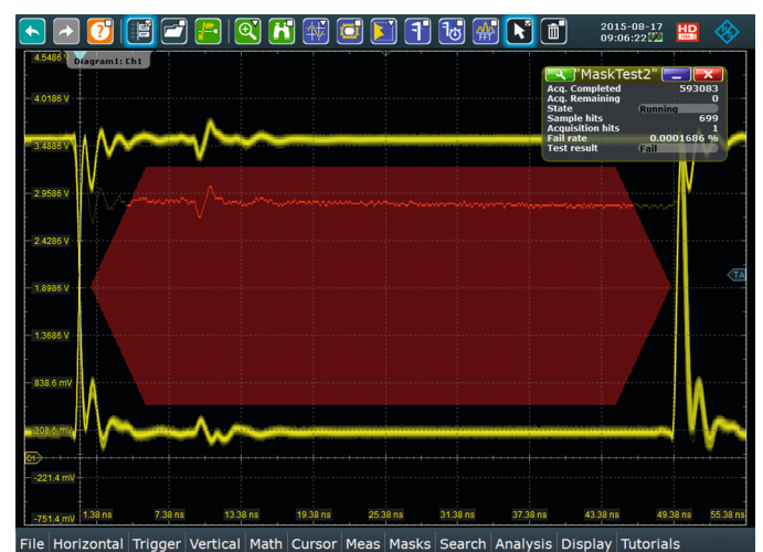
Fast mask test: Within ten seconds, more than six million waveforms are acquired, evaluated and displayed.
