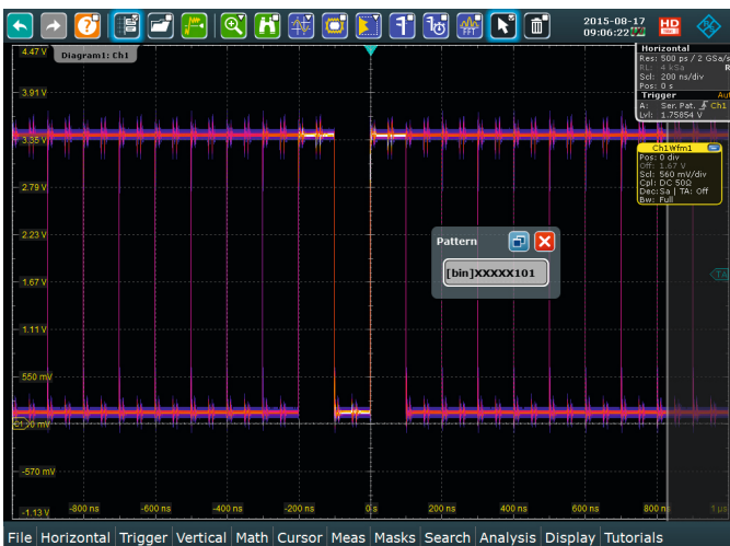
Serial pattern trigger set for a specific bit sequence with the R&S®RTO-K13 clock data recovery option.
