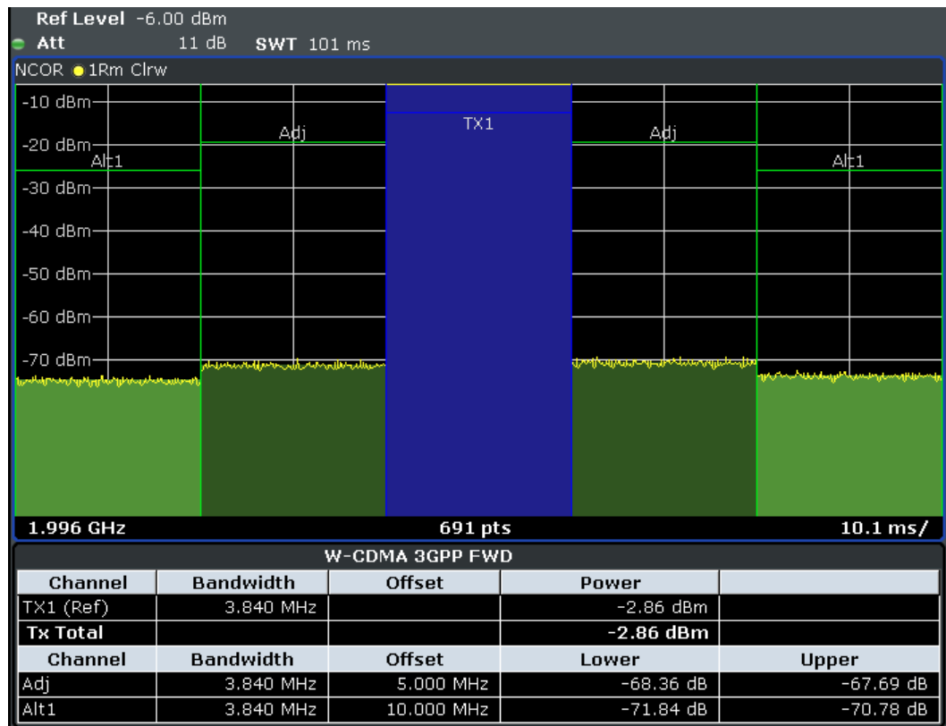
Figure 4-37: Measuring the adjacent channel power of a W-CDMA signal with the fast ACLR mode
