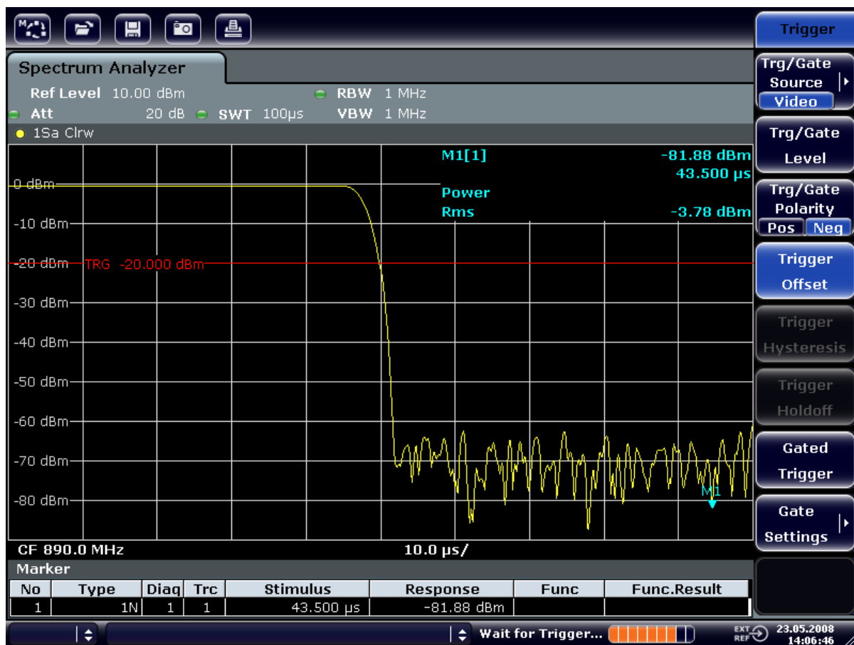
Figure 4-20: Falling edge of the GSM burst displayed with high time resolution
