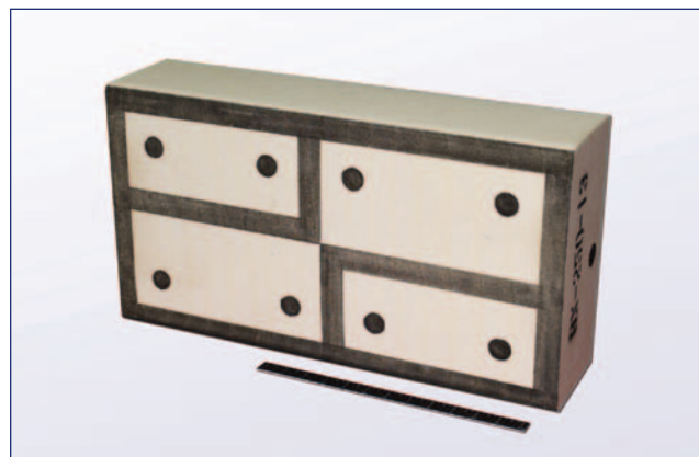
Figure 3.8-3. A typical foam projectile, which has marks for determining position and velocity as well as blacked outlines for indicating the impact footprint.
