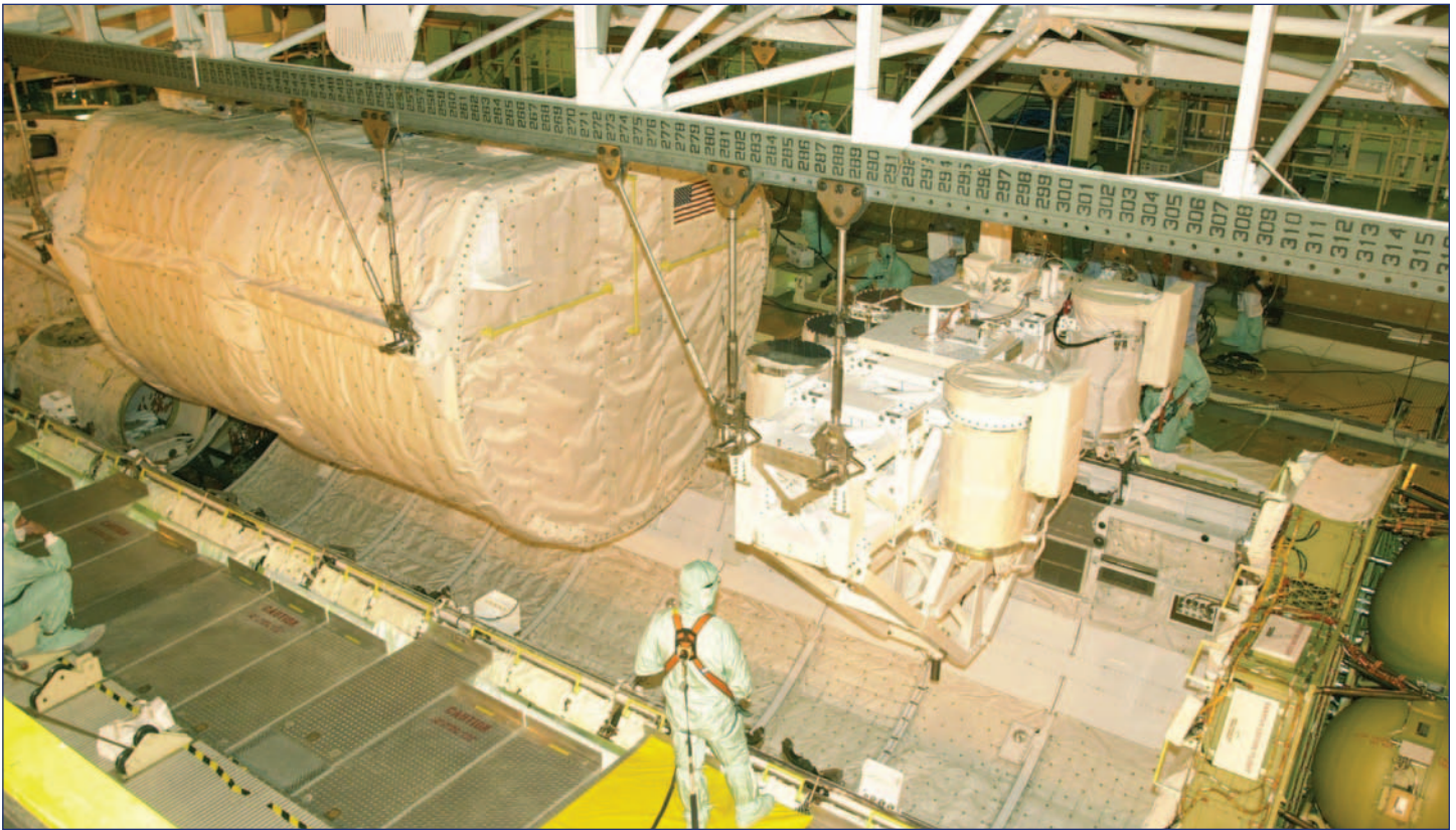
(Above) The SPACEHAB Research Double Module (left) and Hitchhiker Carrier are lowered toward Columbia's payload bay on May 23, 2002. The Fast Reaction Experiments Enabling Science, Technology, Applications and Research (FREESTAR) is on the Hitchhiker Carrier.
