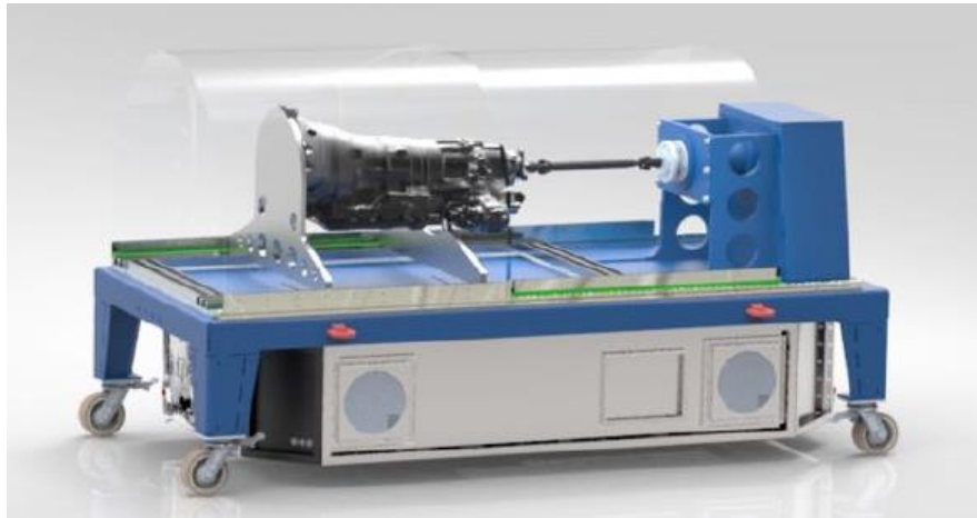
<Mobile EMC motor test bench "BlueBox">
