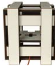
Triaxial Helmholtz coil HCST_50/28_TAP
