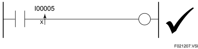
Figure 2.12.6 UPX Allowed Position of AND
