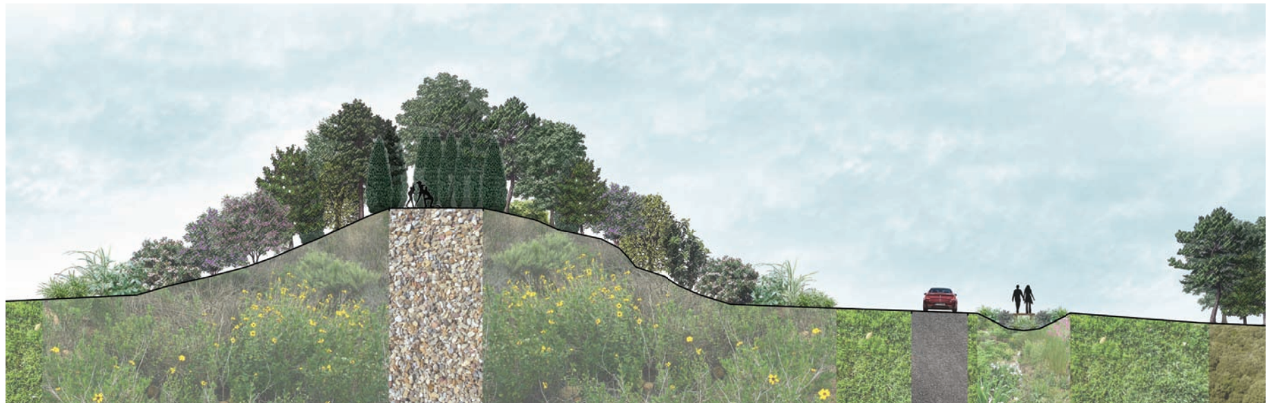
SECTION ILLUSTRATING REVEGETATED WILDLIFE HABITAT ON BUNKER HILLSIDE WITH SECLUDED SEATING AREA AND BIORETENTION SYSTEM WITH RAISED BOARDWALK
