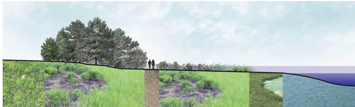
SECTION ILLUSTRATING THE NATURAL TRAIL THROUGH THE COASTAL BUFFER PLANTING ZONE AND FRINGE MARSH BOUNDARY WITH CURRENT MEDIAN HIGH WATER LEVEL AND 5 FOOT SEA LEVEL RISE. LOWER GROWING NATIVE VEGETATION HAS BEEN SELECTED FOR THE WESTERN BANK OF THE TRAIL IN ORDER TO MAINTAIN VIEWS OF THE WATER. SIGNAGE ALONG THE TRAIL EDUCATES USERS ABOUT COASTAL BUFFERS, HABITATS, AND ECOSYSTEMS, AS WELL AS LOW IMPACT DEVELOPMENT METHODS.
