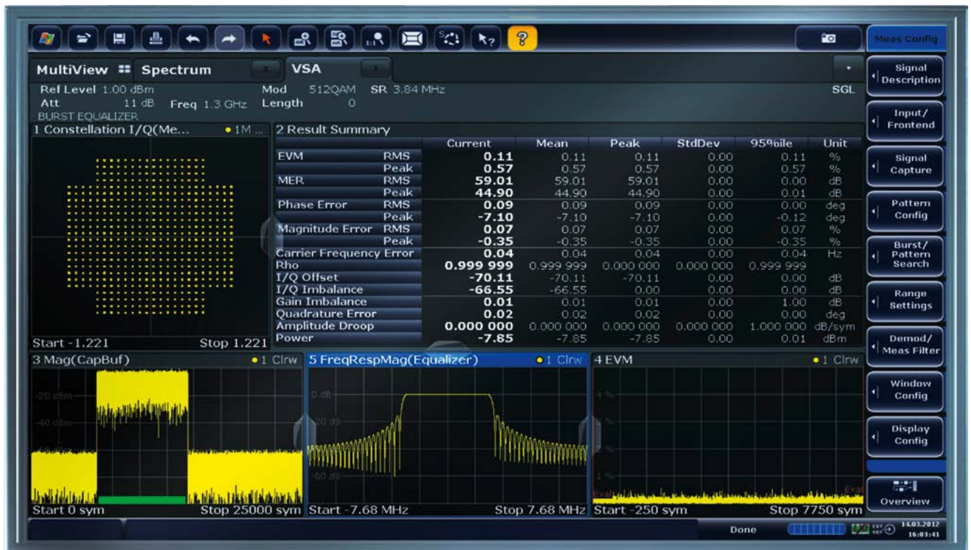
Demodulation of a 512QAM signal with R&amp;S®FSW-K70.
