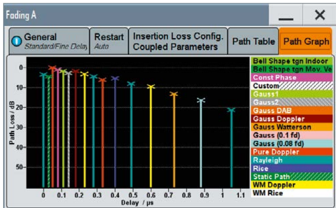
Fading: Power delay profile configuration.
