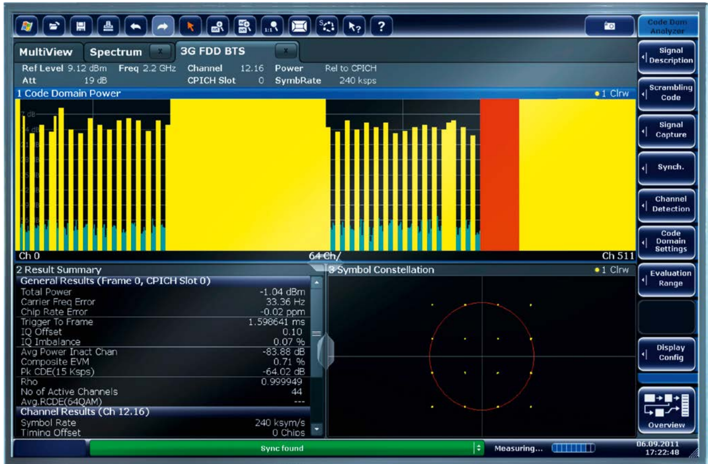
Demodulation of a WCDMA base-station signal with R&S®FSW-K72.
