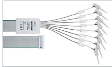
R&S®HO3508 eight-channel logic probe (350 MHz, 4 pF).
