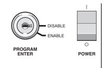
These switches are located in the upper right corner of the front cabinet panel. The key switch is set using the key supplied with the centrifuge; the setting of this switch enables or disables the **PROGRAM ENTER** function. The power switch (30 A circuit breaker) is an ON/OFF toggle switch that, when set to "I", applies power to the centrifuge.
