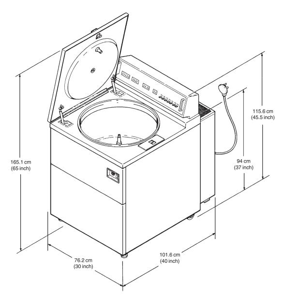
Figure 2-2. Centrifuge Dimensions
