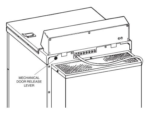
Figure 5-1. Location of Mechanical Door Release Lever
