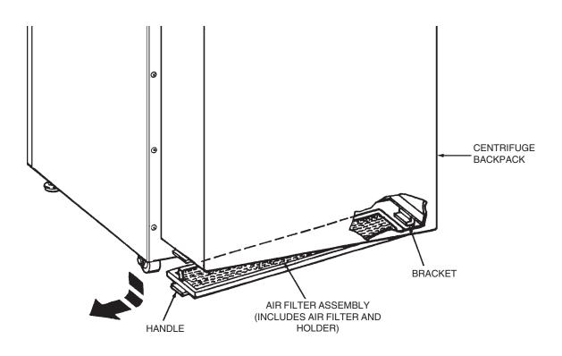
Figure 5-2. Air Filter Assembly Removal
