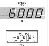
During a run, this display indicates actual rotor speed in rpm (revolutions per minute). If the RPM/RCF switch is pressed to RCF during a run, the display will show RCF (relative centrifugal force) value; if this switch is pressed to PRGM DSPL during a programmed run, the display will show the prerecorded set RUN speed for the selected program.
