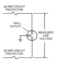
Figure 2-1. RC-3C PLUS Electrical Requirements
