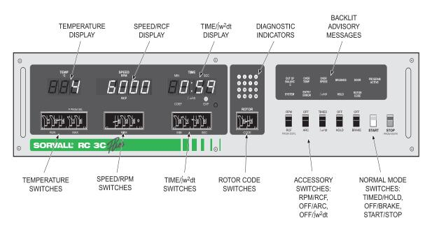
Figure 3-1. RC-3C PLUS Controls, Indicators, and Displays
