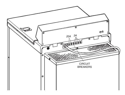
Figure 5-3. Location of Circuit Breakers
