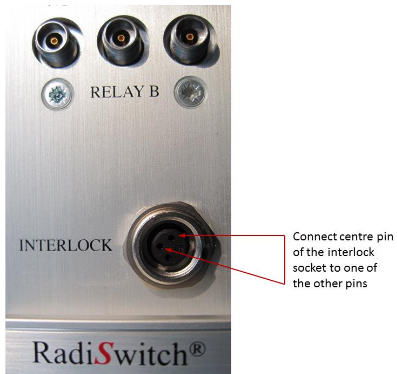
Figure 6: Connector type: Binder 712 99 0405 00 03
